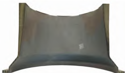
图9 采用优化后浇注系统铸造的机匣试验件剖面图 Fig.9 Section view of experimental cartridge receiver prepared by the optimized pouring system
