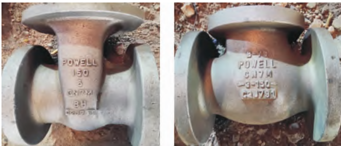
图 7 更改熔炼原材料后生产的精铸件 Fig.7 Investment castings produced after changing the smelting raw materials
