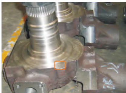
图 8 铸件加工后缺陷部位 Fig.8 Casting defects after machining
