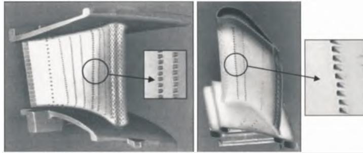
图1 发动机涡轮叶片表面的气膜冷却孔<sup>[6]</sup>Fig.1 The film cooling holes (FCHs) on the surface of the engine turbine blades<sup>[6]</sup>
