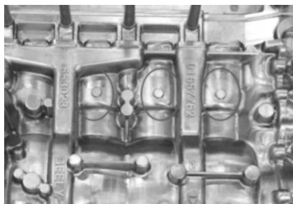
图2 模板上用于在铸型中形成凹坑以定位芯撑的凸台 Fig.2 Small bosses on the pattern plate to form pits in mold to position chaplet
